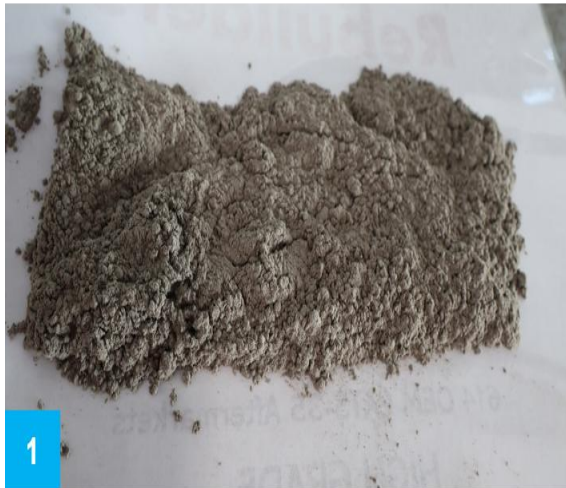
Figure 2: 1. Pulverised spent catalytic converter; 2. Conventional flowsheet for catalytic converter processing (Yakoumis, I., et al. 2021)
