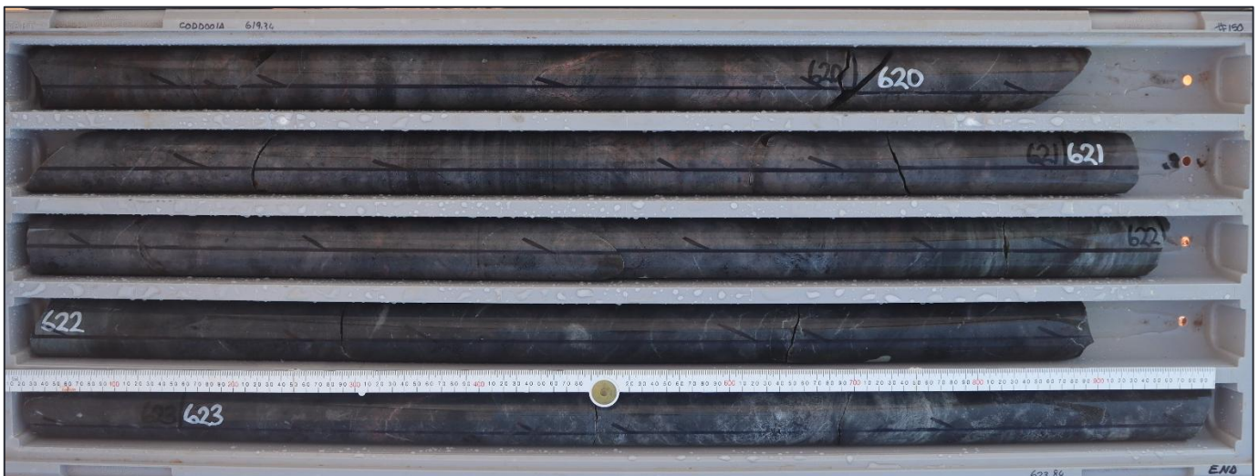
Figure 3: Core tray photo from Coogee North hole CODD001a, highlighting the typical brittle deformation and associated hematite-silica alteration (note ruler for scale).
