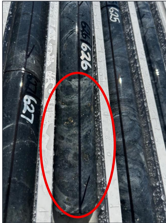
Figure 4: Example of trace disseminated sulphides (pyrite/chalcopyrite) in deformed and altered intermediate volcanoclastics from Coogee North hole CODD001a, at 626.0 – 626.3m downhole.
