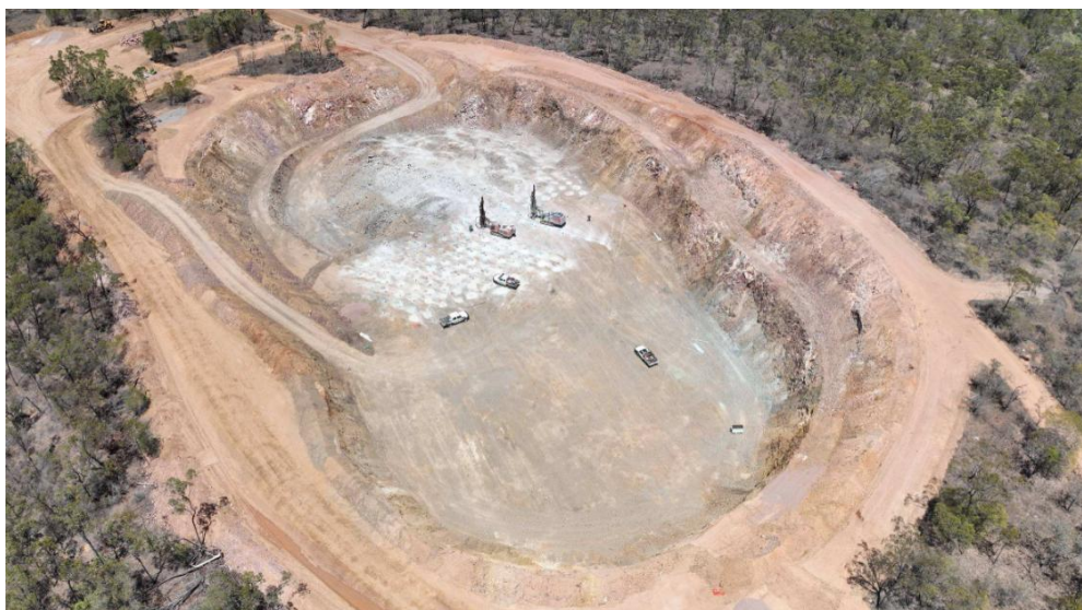
Figure 3: Podosky mining area showing the 257.5 RL bench at approximately RL265 following latest blasts. Mining is scheduled to be recommenced on 2 October 2026.
