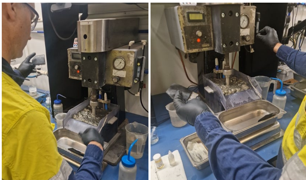
Figure 3. Southwest rougher flotation test work trials.
