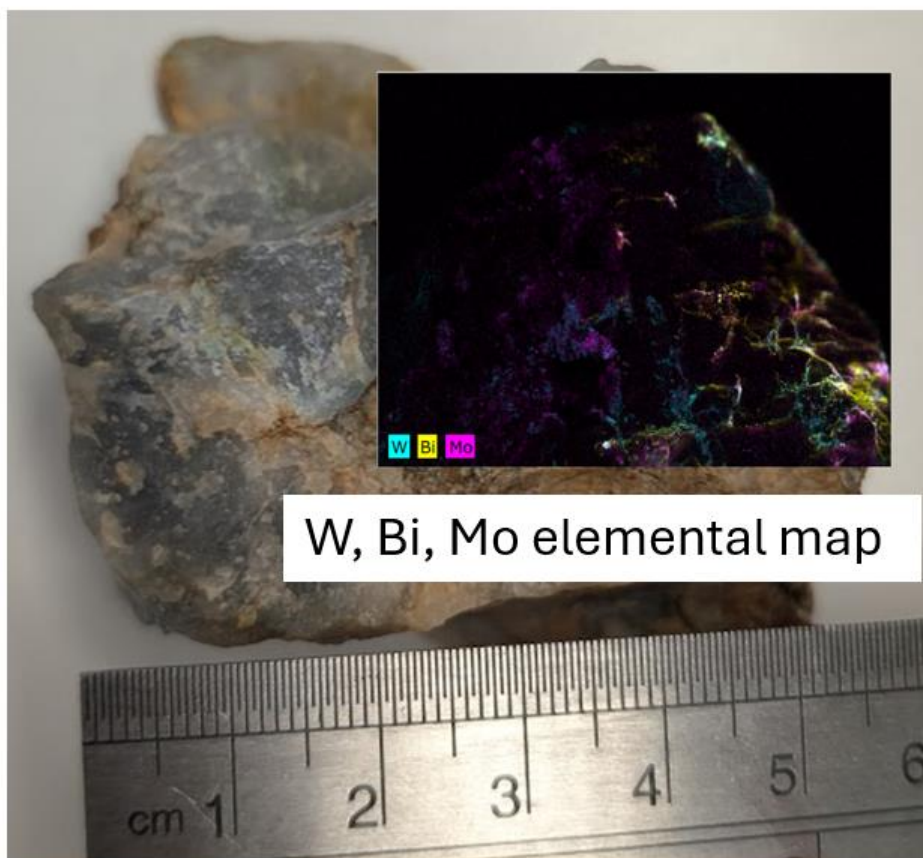
Figure 5-7: Hand specimen (SY09) showing the micro-XRF scanned area (red rectangle) and accompanying W, Bi and Mo and Cu maps. Maps show relative X-ray counts (qualitative).
