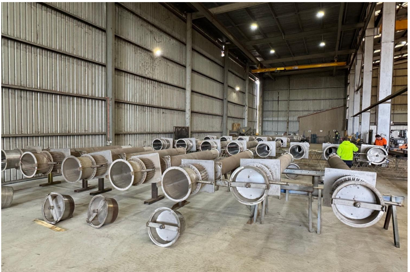
Figure 8: Vacuum testing of condenser and retort assemblies
