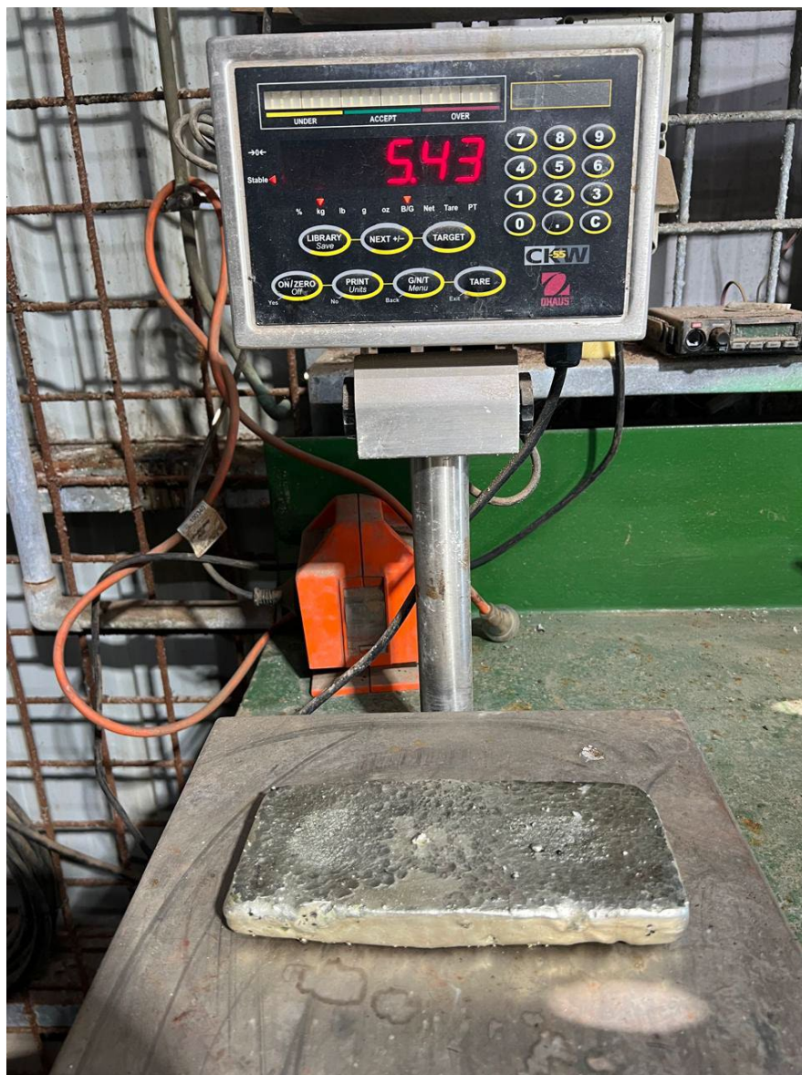
Figure 1: Doré bar PGO-03 weighing 5.43kg with an estimated 70:30 gold to silver ratio
