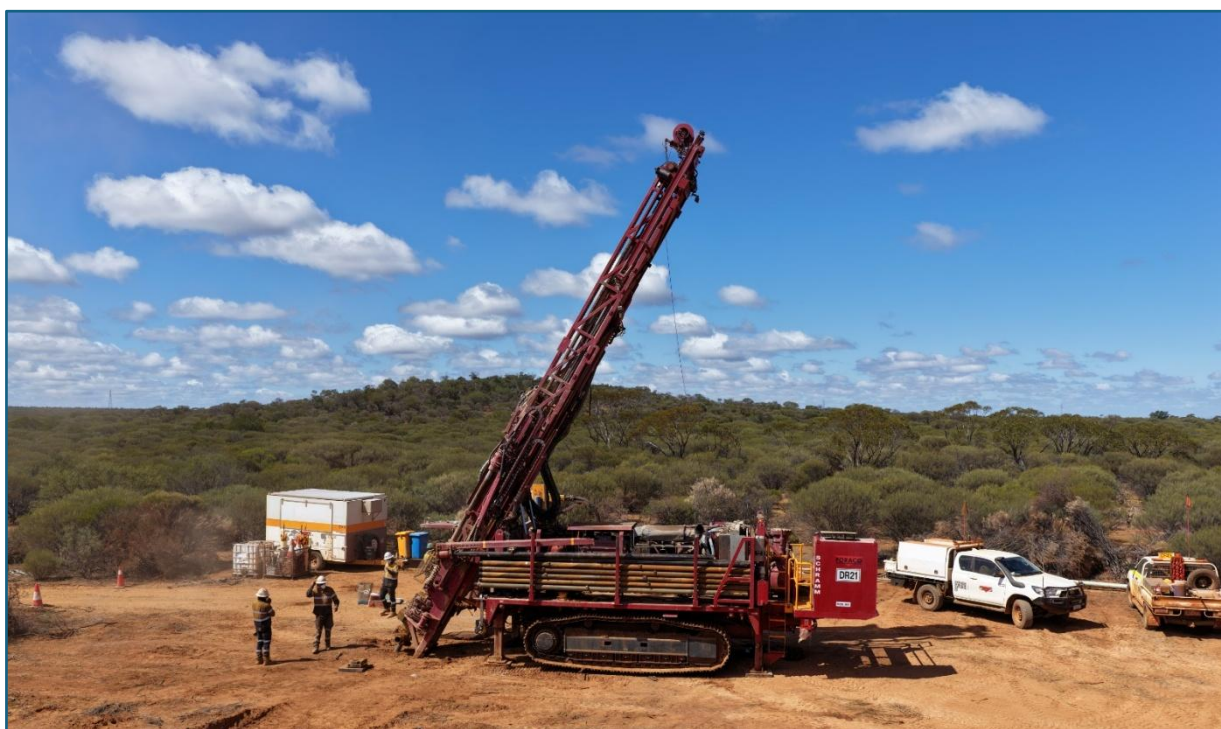
Figure 1: Photo of RC drilling at Killi Resources' Lodestone Iron Ore Project
