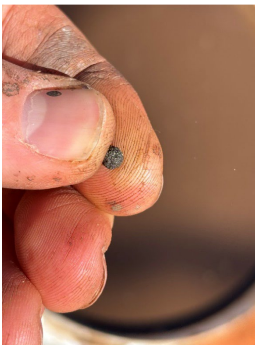
Figure 8: Typical example sulfide nodules from sieved sample at Hatlifter
