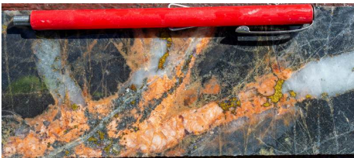
Figure 3. Mineralised volcanic sediments from 373.6m depth in hole BD019003, Briggs Central. Within a 1.05m sample which assayed 0.39% Cu. Core diameter 61mm.
