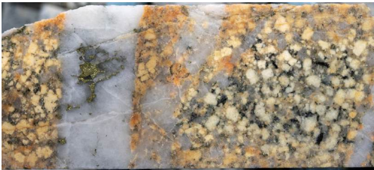
Figure 2. Mineralised porphyritic granodiorite from 134.7m depth in hole 25BRD0037, Briggs Central. Within a 2m interval which assayed 0.53% Cu. Core diameter 61mm.
