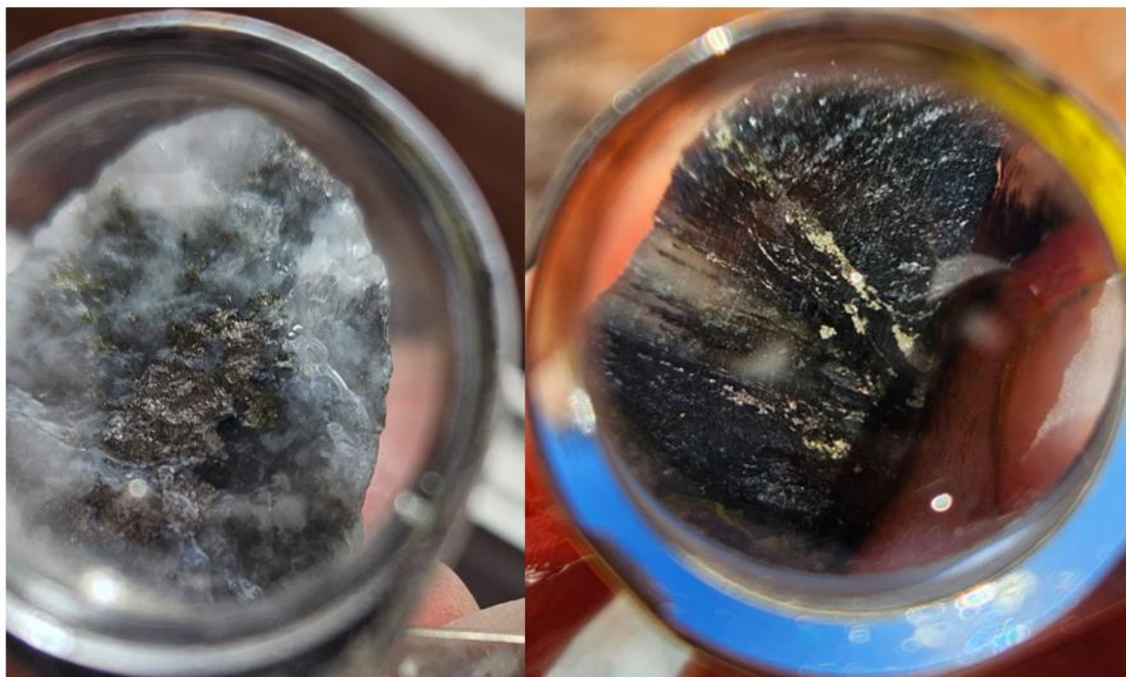
Figure 3: Left hand image taken from 170-171m in hole 26ANRC012 shows 2 species of sulphides with the brassy looking one pyrrhotite and the most yellow one pyrite visual estimates are 1% for both pyrite and pyrrhotite in this interval. The Right hand image shows sheared fine grained, black mafic unit (basalt or chilled margin) with sulphides on both the primary shear fabric and filling cross cutting fractures from 226-227m in hole 26ANRC011 with visual estimates for pyrrhotite of 0.2% and 0.1% for pyrite 1 and 3 .
