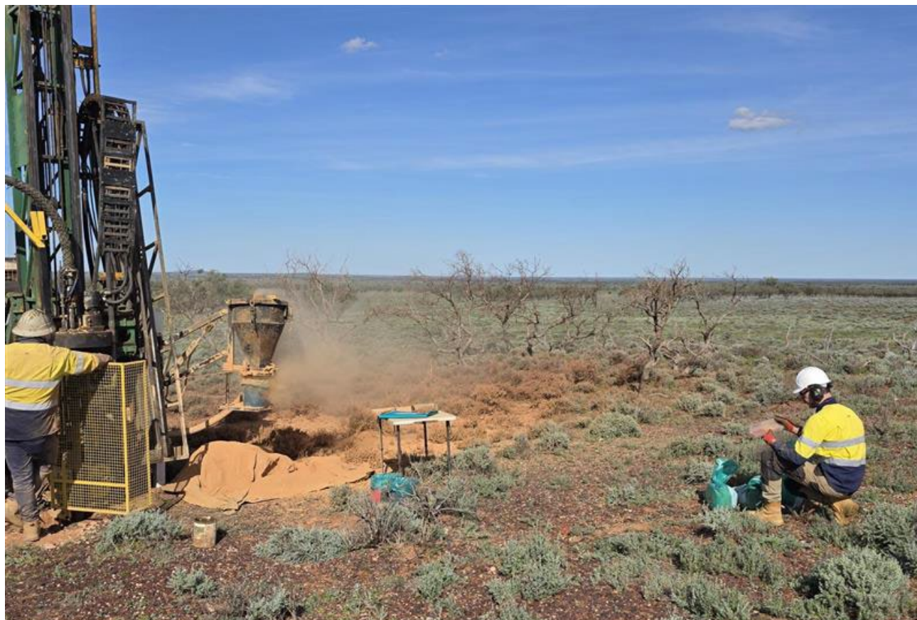
Figure 1. Air core drill rig, drilling at the Ironback Hill REE Prospect
