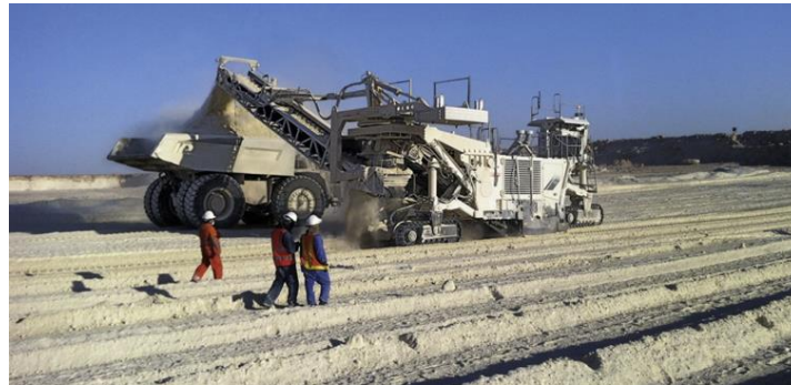
Fig 2 – Surface Miner – Limestone row cutting and simultaneous direct truck loading
