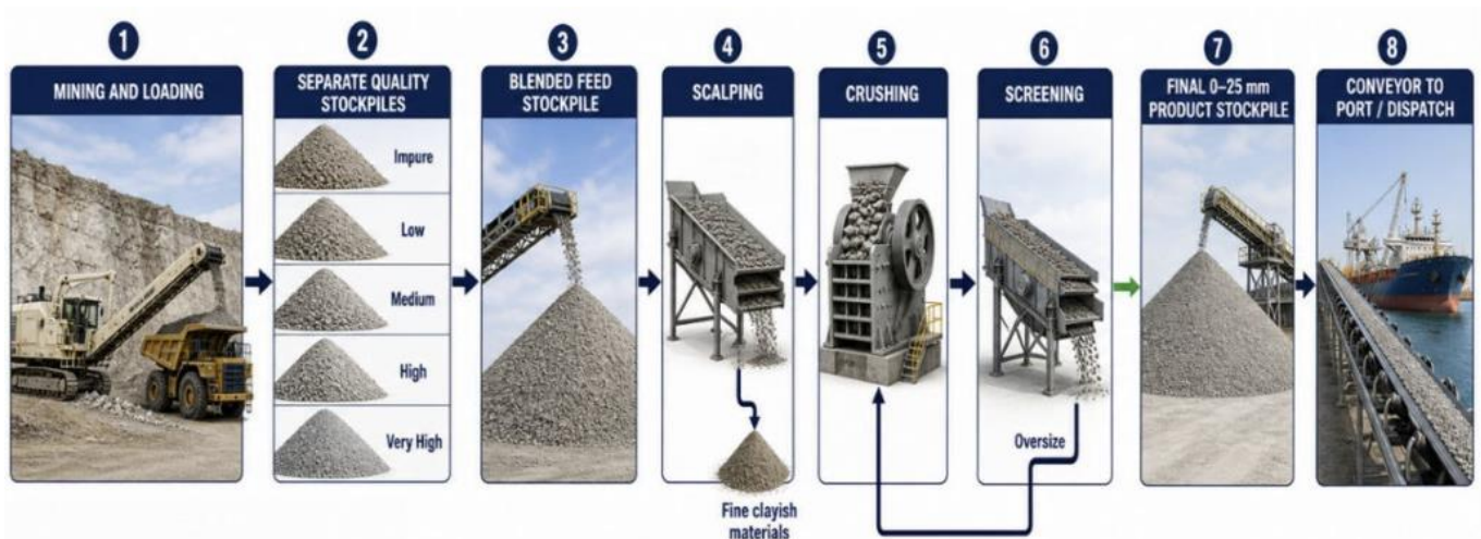
Fig 4 – Limestone Processing Flowsheet (nominal sub-25mm shown)
