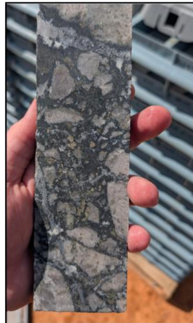
Figure 6: Mineralised drill core, hole MMDD007 (171m) - enargite-pyrite hydrothermal breccia.
