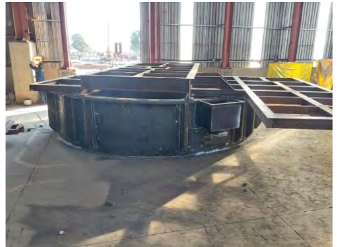
Figure 9: CIL Tank fabrication
