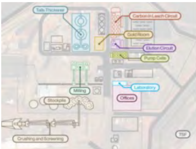
Figure 4: TGME Gold Project Processing Plant (Plan View)
