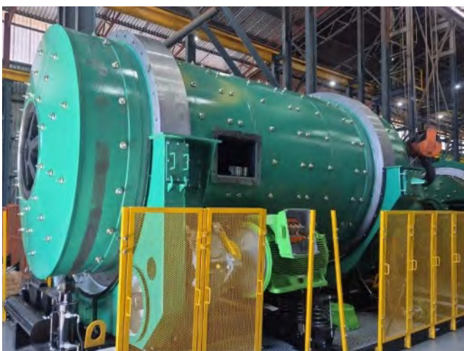
Figure 10: Ball Mill - complete shell, feed/discharge ends, drive interface
