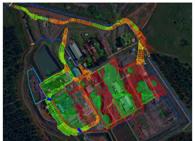
Figure 11: Bulk Earthworks cut and fill requirements (Red area to be cut and Green to be filled)
