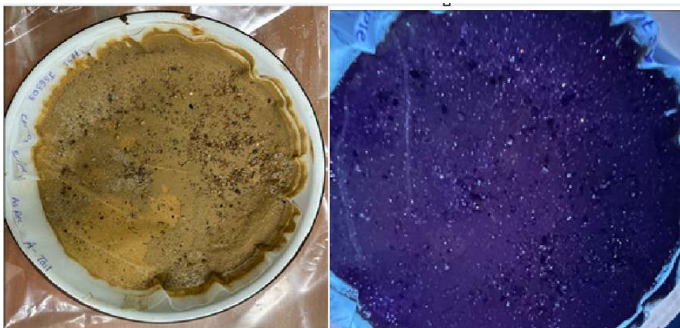
Figure 5. Kookynie Tailings - Knelson gravity concentrate under natural and ultraviolet light, showing fluorescent scheelite.
