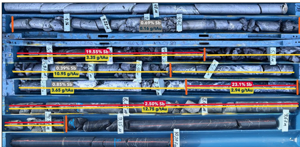
Figure 4: Drill hole UG25ZOP003 mineralised core showing significant gold-antimony intersections
