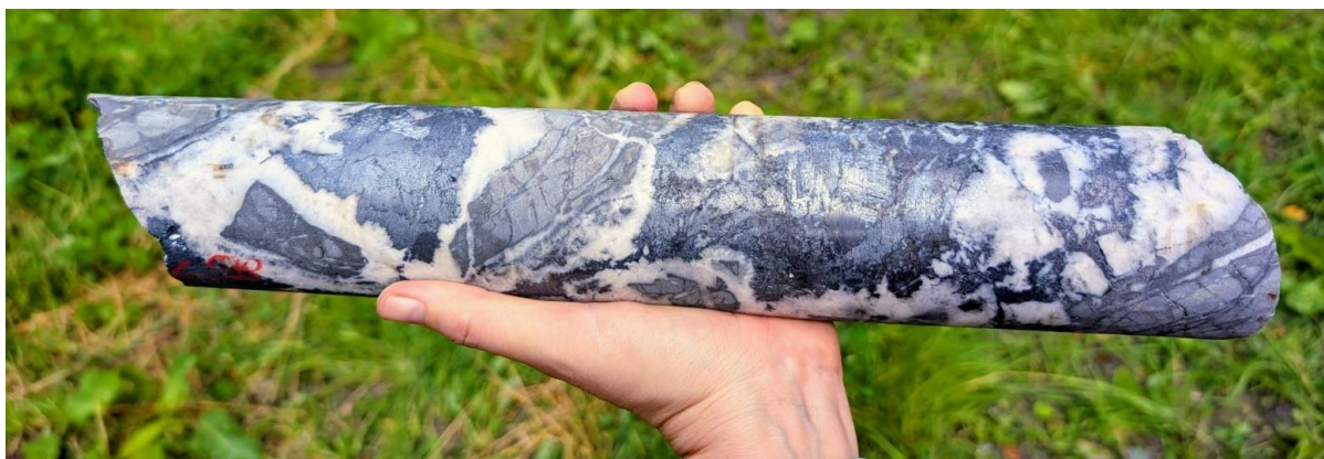
Figure 6: Photograph of 44cm long drill core from hole DD26ZOP-002 (interval 44.66 – 45.00m) showing stibnite (antimony mineral) (estimated ~25%), slate and quartz breccia with disseminated sulphides. Assays were pending at 30 June 2026.
