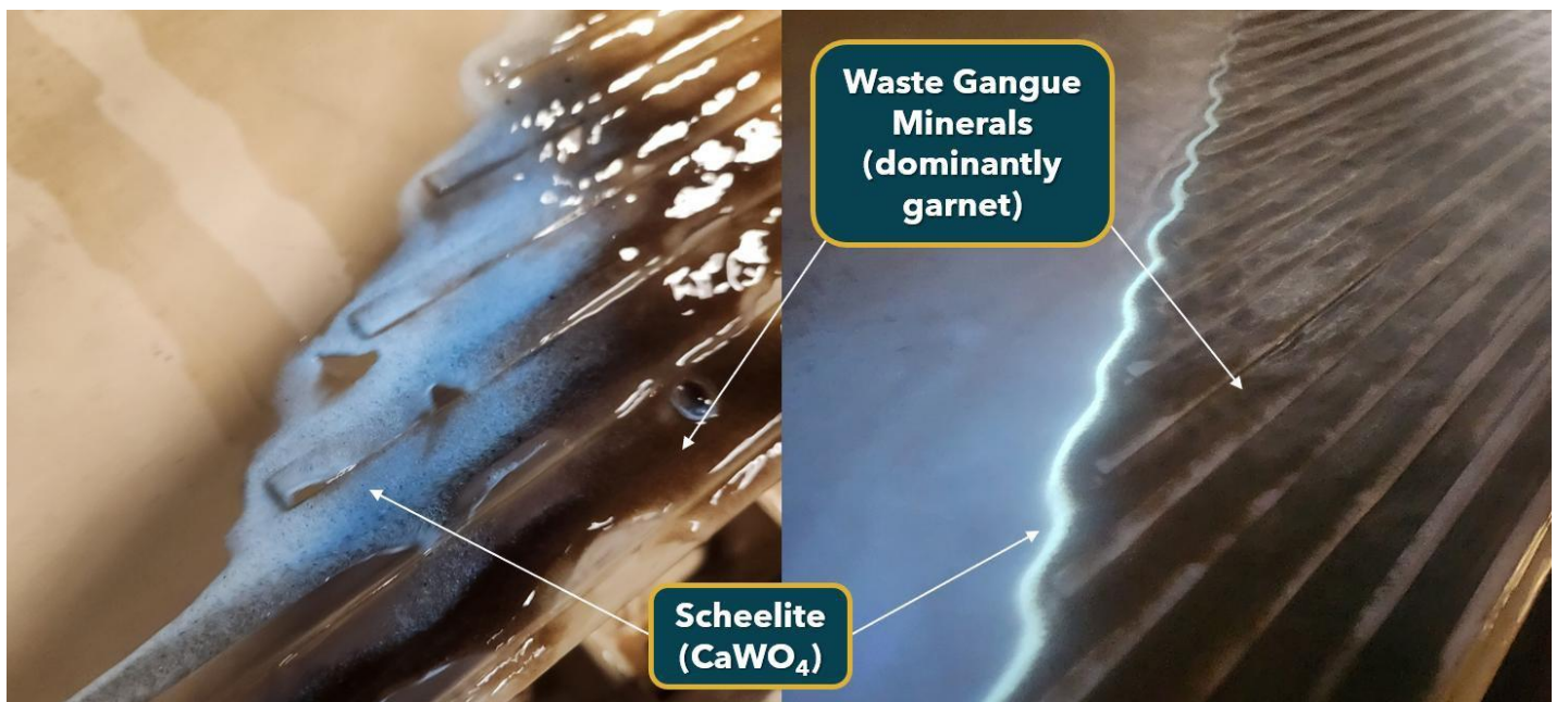
Figure 8: Scheelite separation on the Wilfley gravity table during testwork on Linka mineralisation
