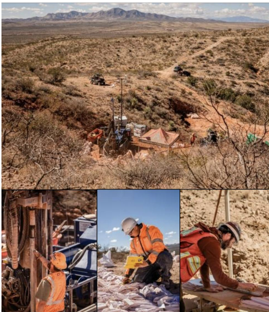
Figure 3: Clockwise from top. Midnight Sun's Grasshopper RC rig drilling RBRC026. Company geologist inspecting RC chips. Field technician collecting magnetic susceptibility measurements. RC drilling rod change.
