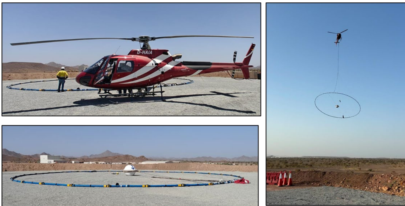
Figure 5 – HeliTEM Airborne Electromagnetic Survey in Action
