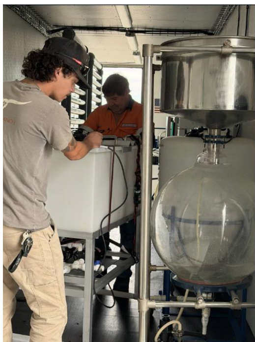
Figure 11: Greg and Preston setting up the Iron removal equipment
