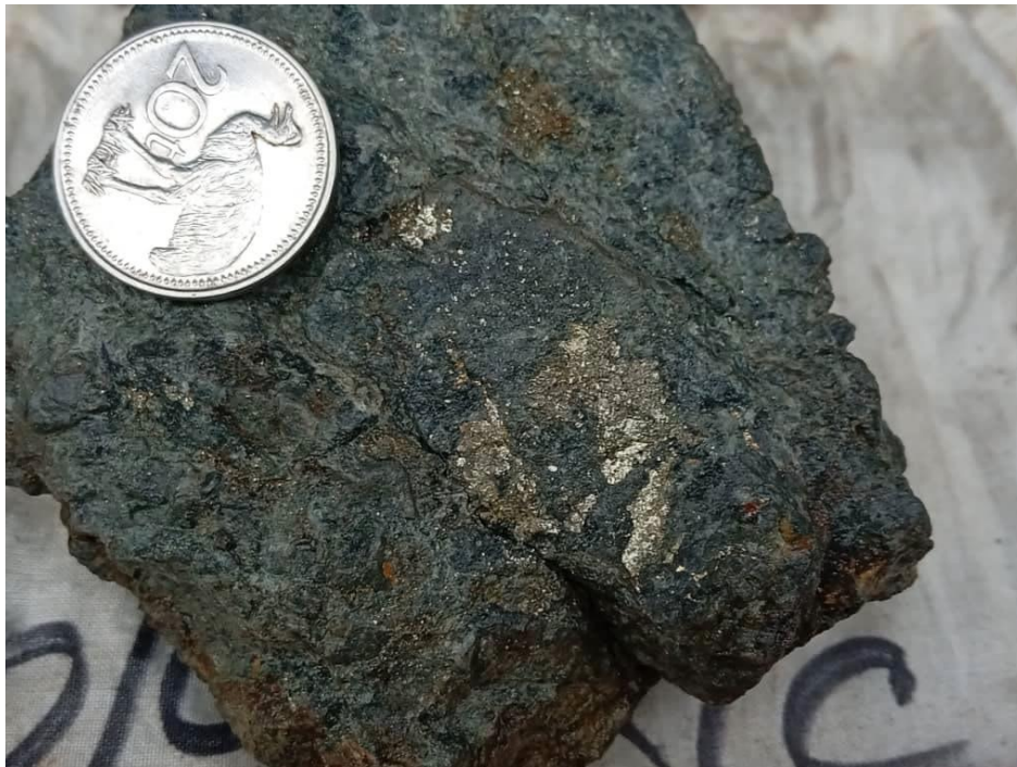
Figure 8: Outcrop Sample 702110 – Visible sulphides in breccia of andesitic volcanic sediment from North access track to Agadul. Visual estimate of sulphides 3% pyrite and 0.5% of fine chalcopyrite 11
