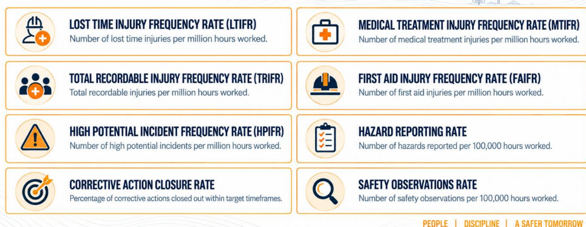
Figure 23 Proposed safety KPI framework covering injuries, high-potential incidents, hazard reporting, corrective-action closure and proactive safety observations.
