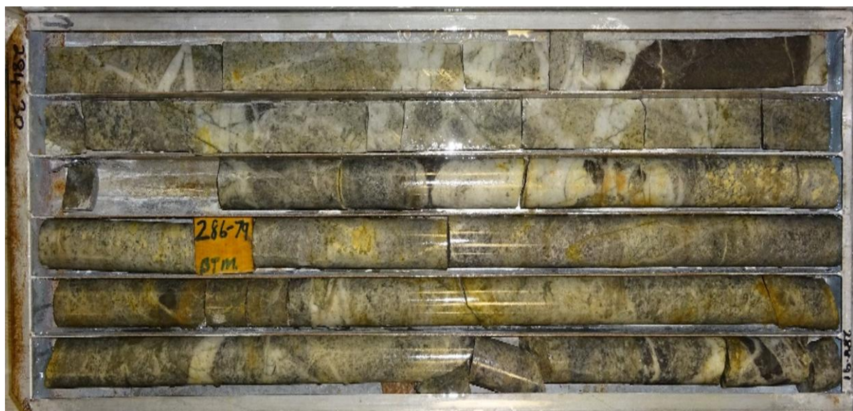
Figure 12. Hole NS4 intersected stockwork porphyry mineralisation at 280m depth, which confirms the exploration model.
