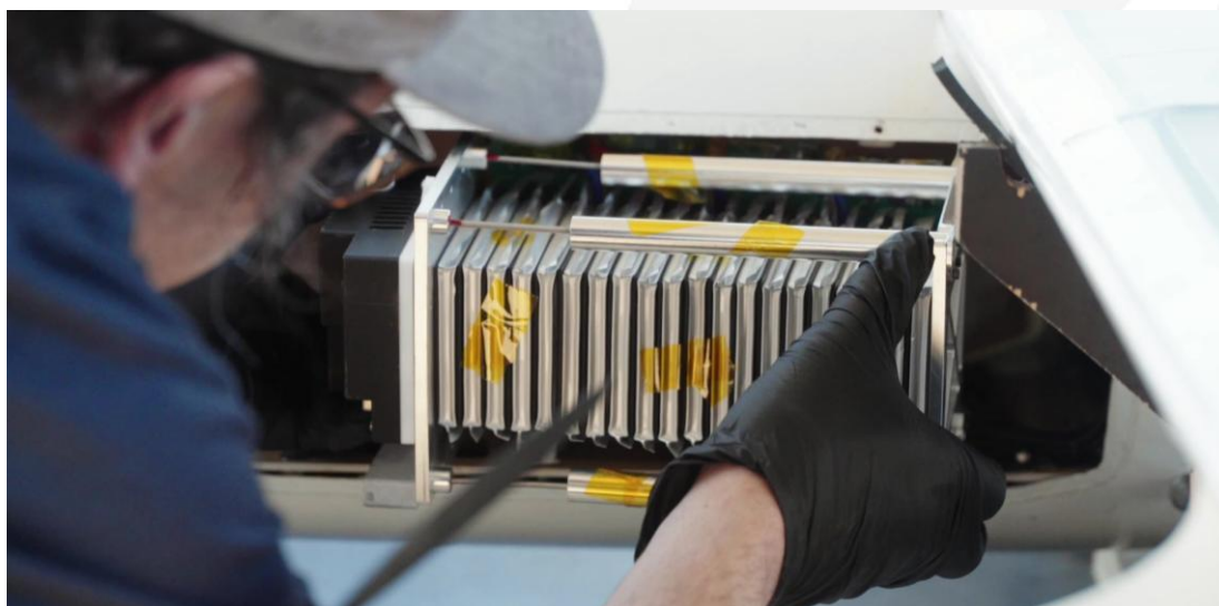
The Li-S Energy lithium sulfur battery pack being installed in the Pegasus fuselage ahead of flight testing
