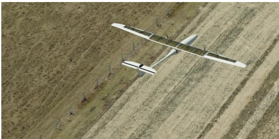
The EATP Pegasus in flight over Queensland, with the Halocell perovskite solar arrays visible along the wings
