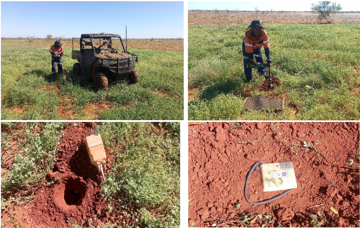
Images: Passive seismic nodes being positioned for data collection as part of 2026 Passive Seismic Survey
