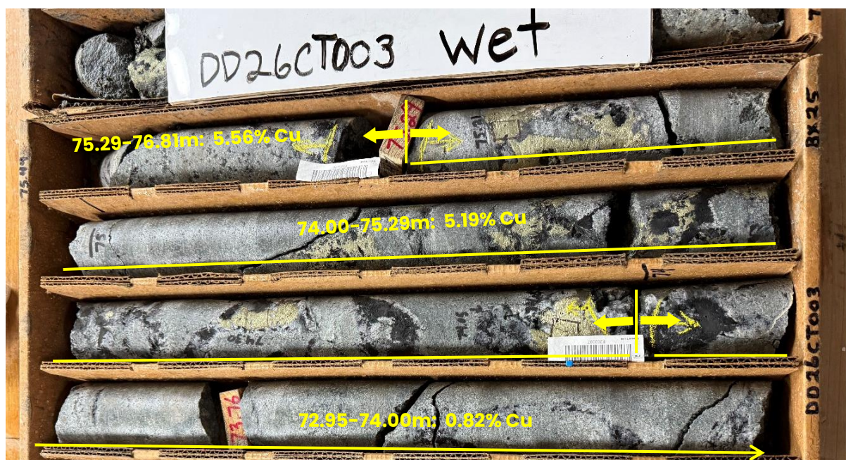
Figure 4: Copper mineralisation and lab assays down Cactus Corridor hole DD26CT003.
