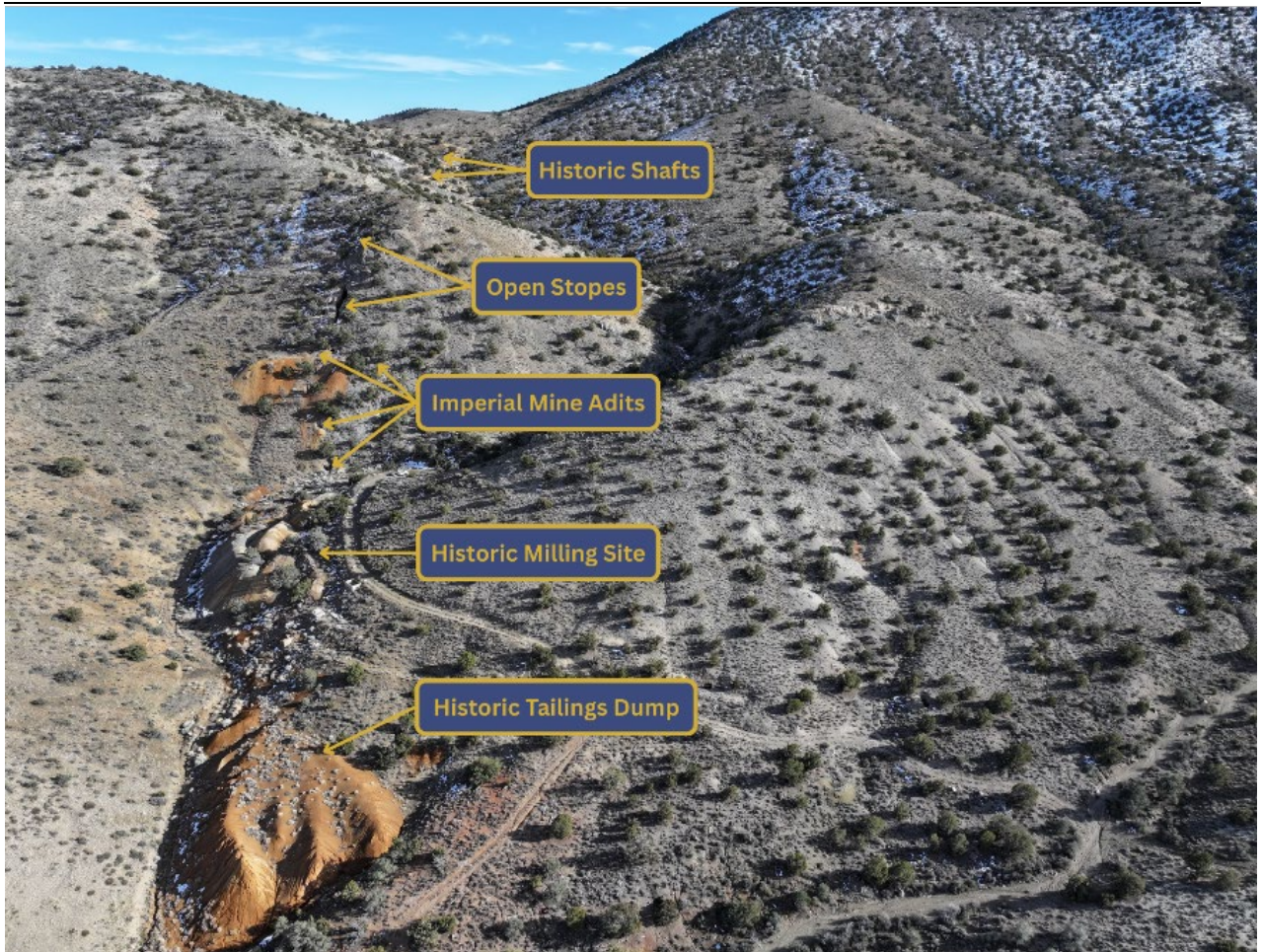
Figure 3: Oblique view facing south of Imperial mine showing workings and historic infrastructure
