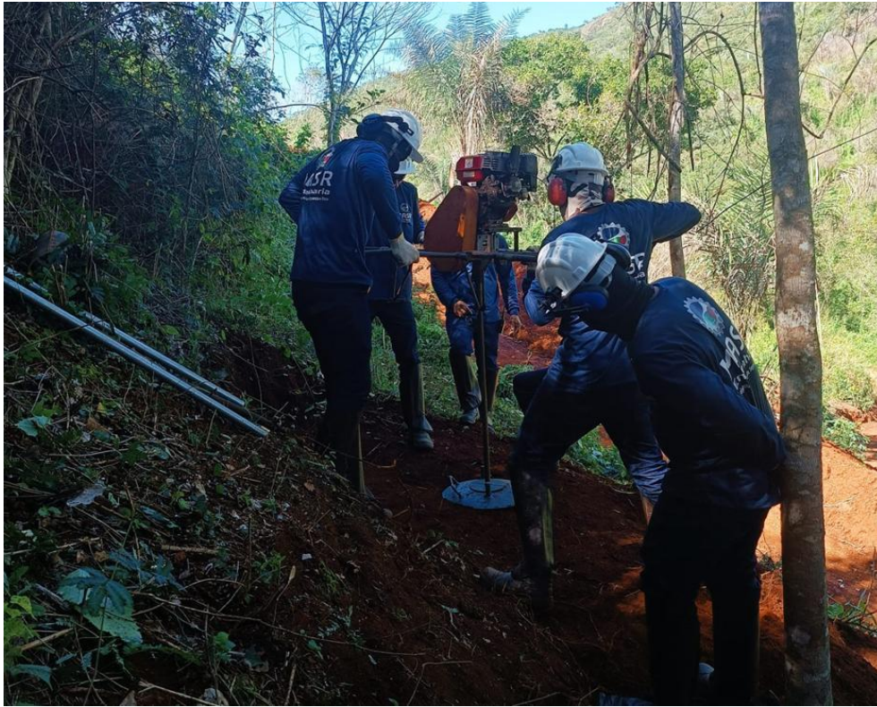
Figure 4: Auger drilling underway at Eminence Minerals' Campo Grande Project, Bahia, Brazil.
