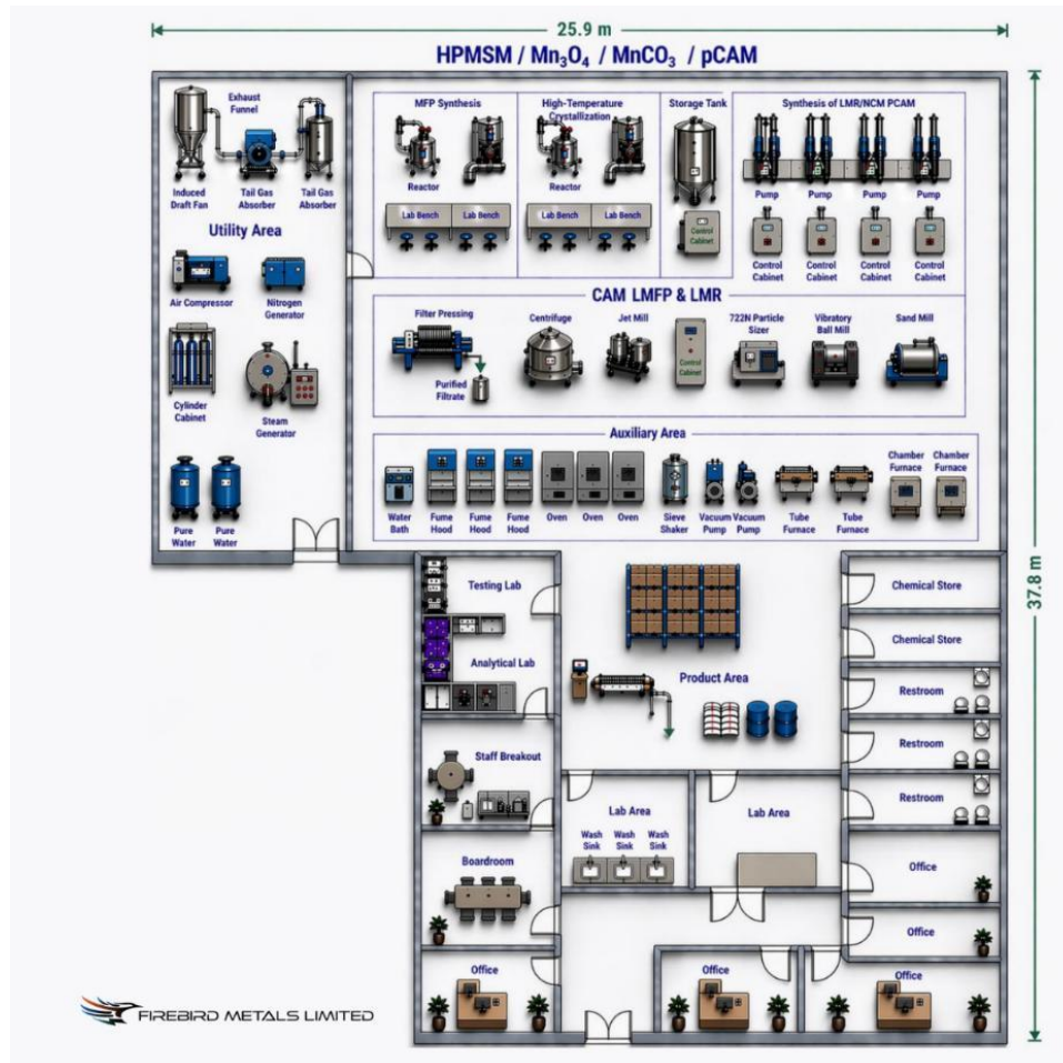
Model diagram and layout of the proposed Australian Demonstration Plant, Osborne Park
