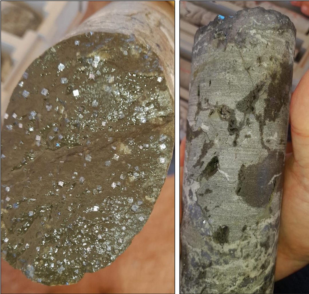
Figure 8-4: Sorby Hills – visible galena in the core (on the left) and porous core (on the right)
