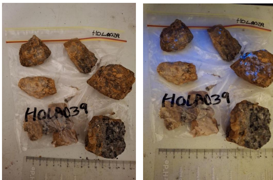
Figure 4: Sample HOLA039 grading 12.45% W (15.69% \text{WO}_3 ) – under normal (left) and UV(right) light
