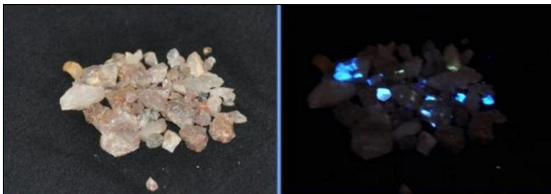
Figure 2: Sample MPL21_559 under natural (left) and UV (right) light highlighting scheelite (tungsten) luminescence.
