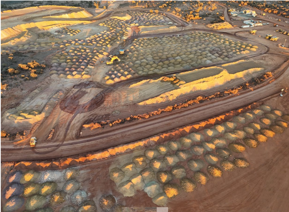
Figure 3. Individual truckloads free dumped at the re-handle stockpile areas, 31 August 2026
