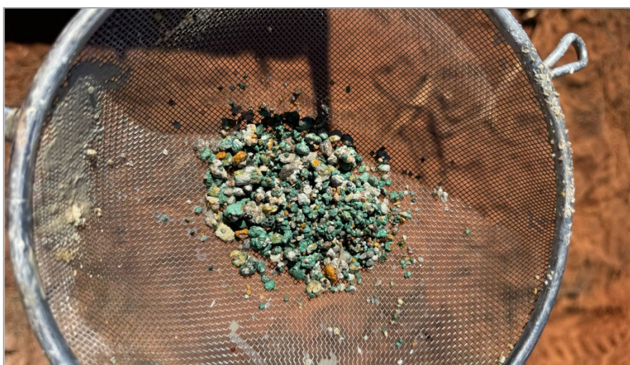
Photo 1: Recent drill hole EPT 2439 Copper Oxide Mineralisation (Malachite) at 46-47m (part of 2m @ 1.7% Cu) 6
