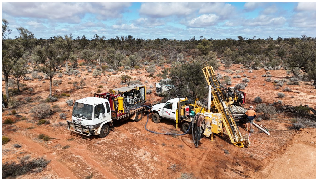
Figure 5: Aircore Drilling at Tunkillia North
