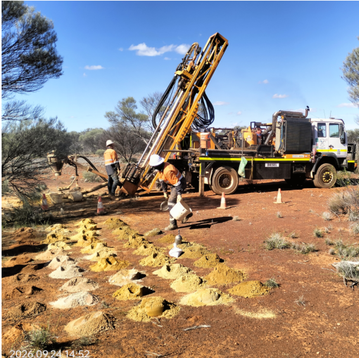
Figure 1, Bostech drilling onsite at KGP with aircore rig
