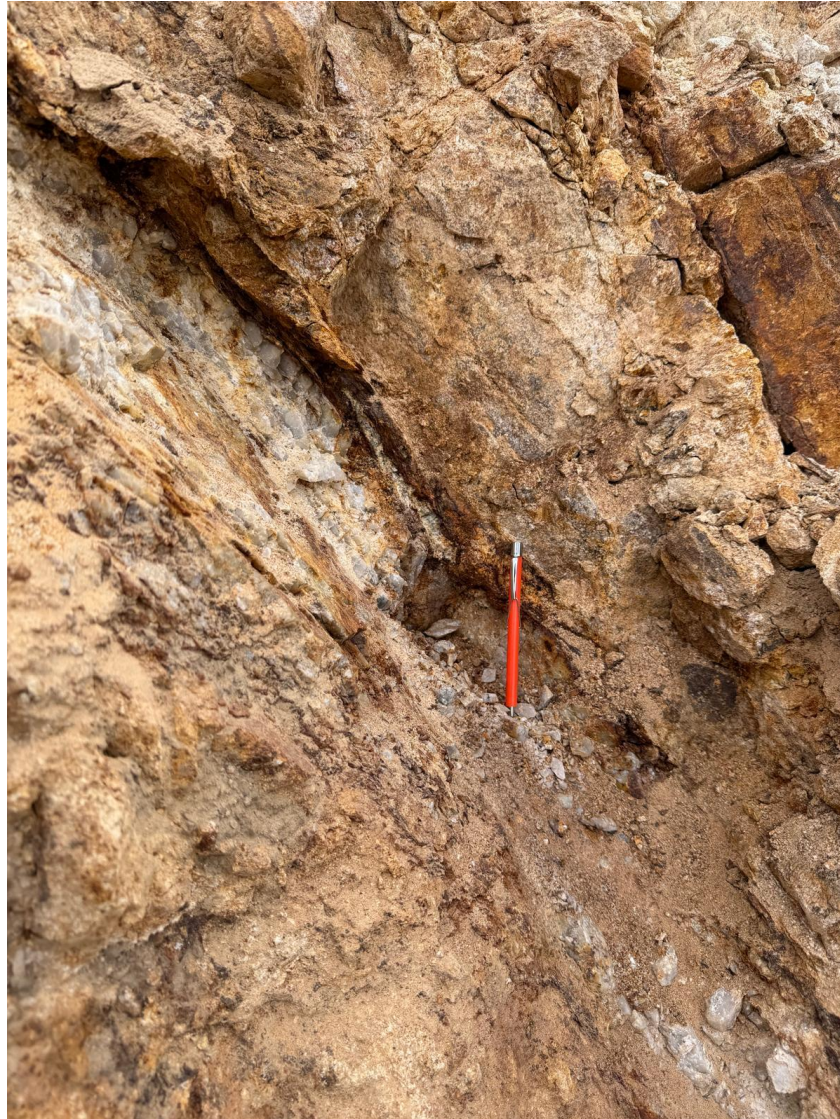
Figure 8: Stringer vein, approximately 20cm in thickness, observed in the face of drill pad cutting. A 3.3 kg sample from this vein returned assay results of 344 g/t Ag and 0.53 g/t Au.
