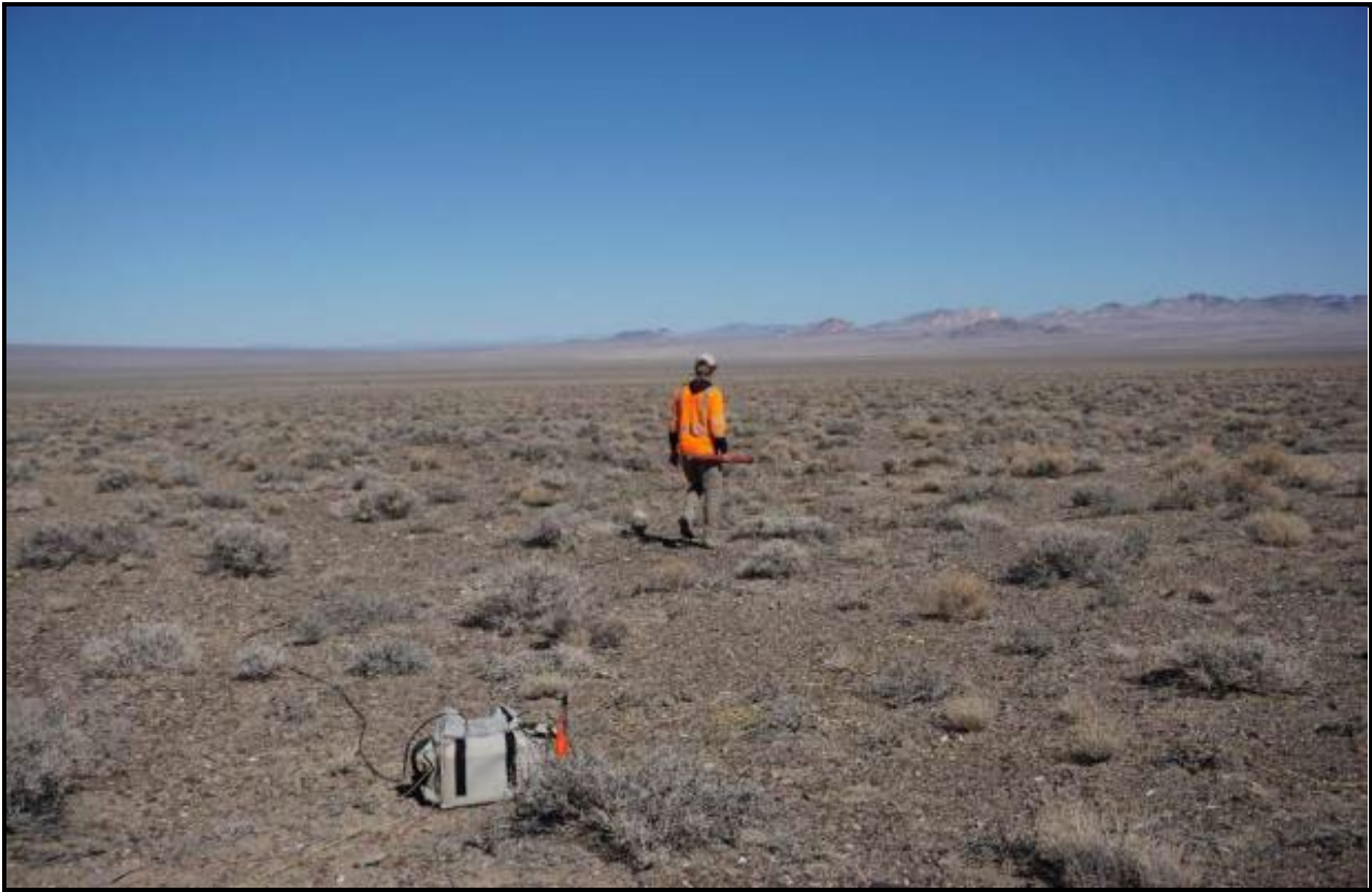
Figure 6. CSAMT SURVEY RECIEVER DEPLOYMENT AT THE ALKALI FLATS PROJECT
