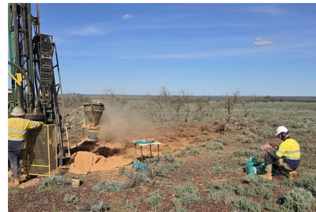
Air core drill rig, drilling at the Ironback Hill REE Prospect
