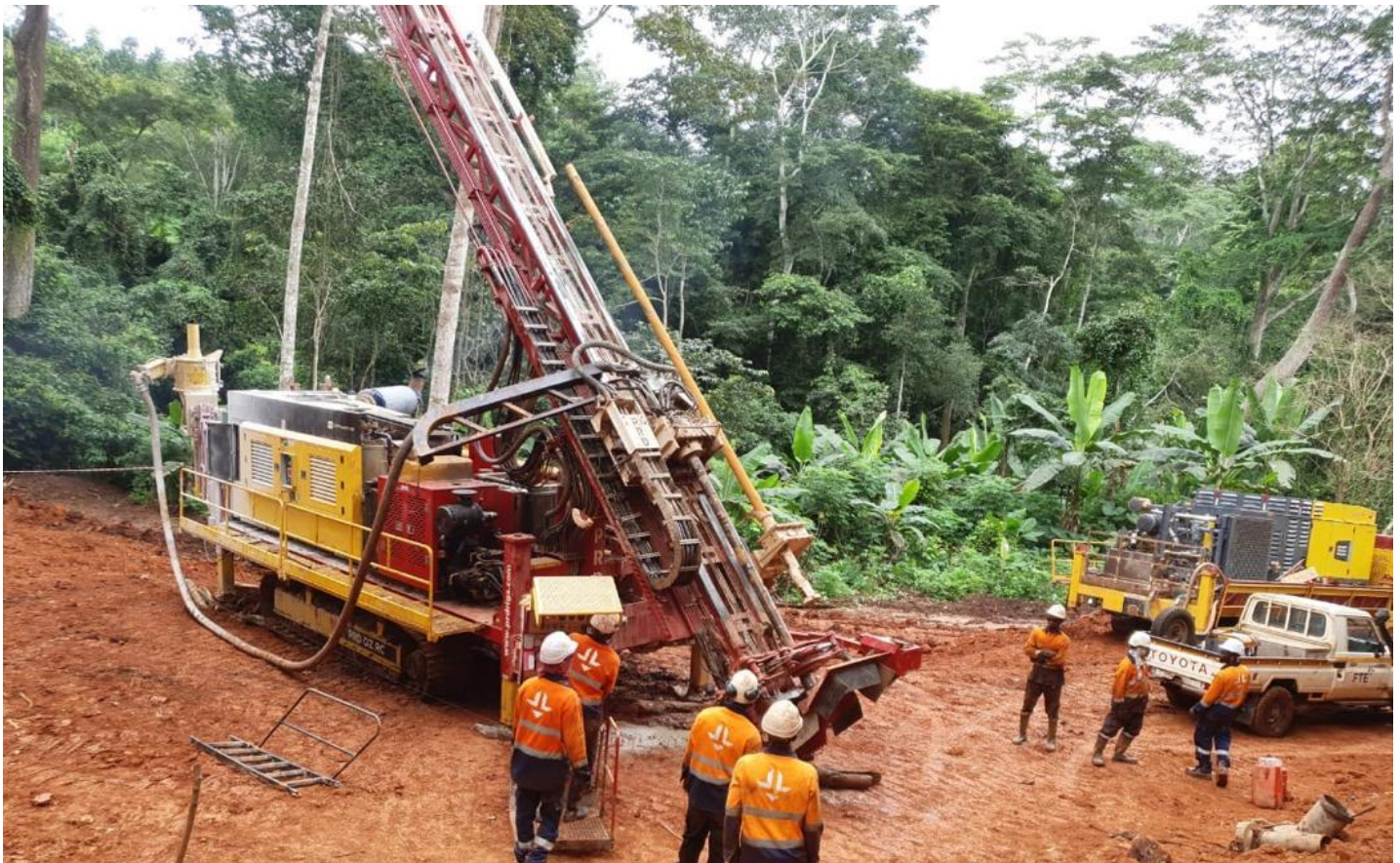
Figure 3. RC drill rig setting up on the second drill hole collar.
