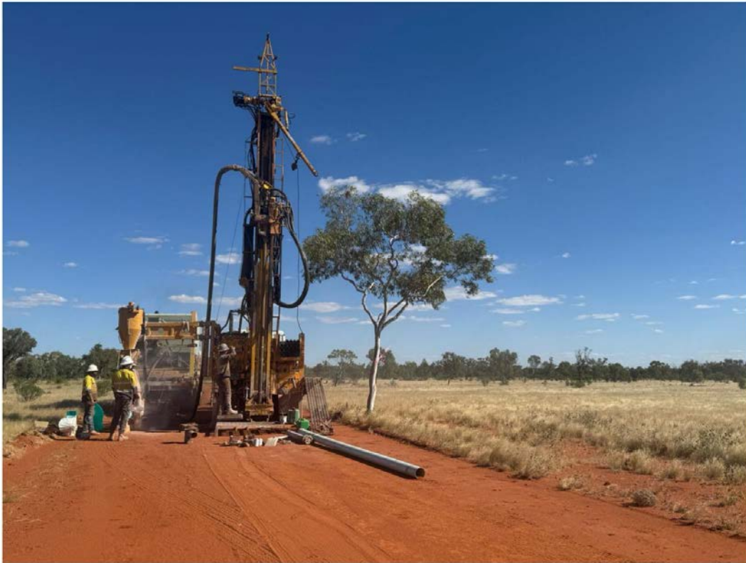
Figure 8: RC drilling underway at the Newmans rare earth prospect, April 2026.
