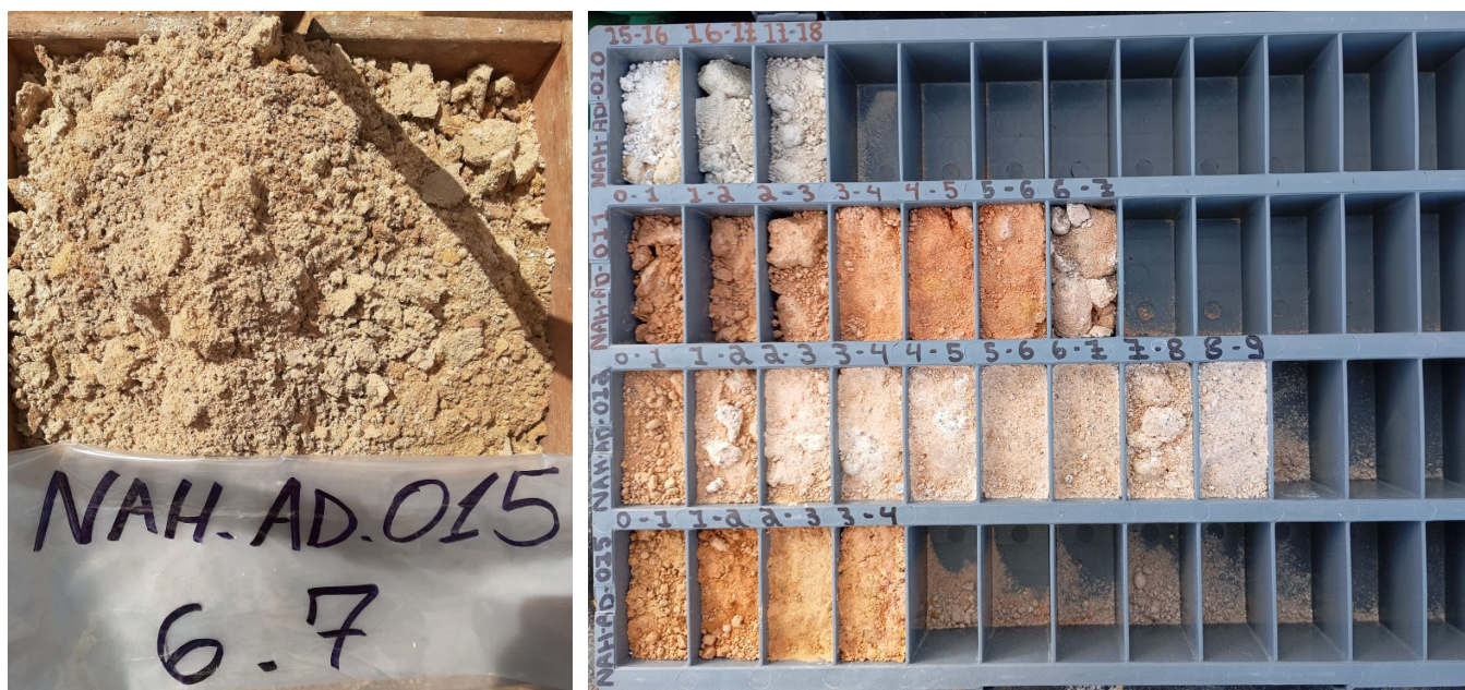
Figure 4A and 4B: Auger cuttings from NAH-AD-0015 being collected and retained in chip trays.
