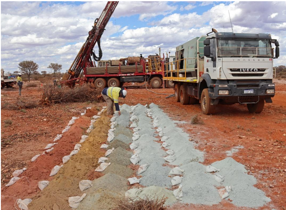
Figure 4: RC drilling of the type completed across Golden Crown, Dumbarton and Sunday Picnic during FY2026.
