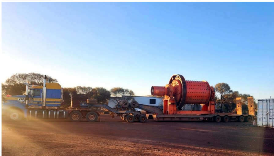
Figure 5: Ball Mill during relocation.
