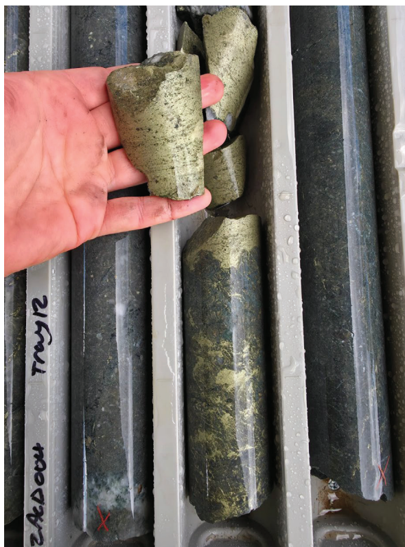
Figure 6: Monza hole MZACD004. Chalcopyrite and pyrite sulphide breccia within potassic altered monzodiorite porphyry. 0.99g/t Au & 4.1% Cu.
