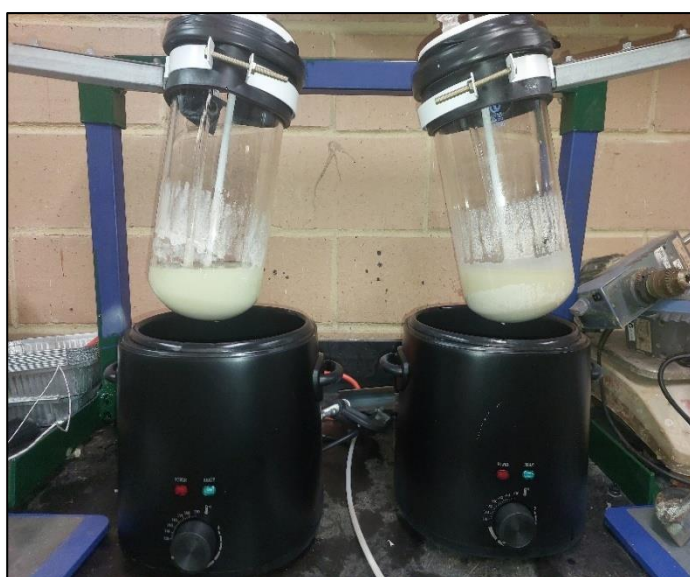
Image 1: Hydrolysis and precipitation of titanium in stirred glass reactor.
