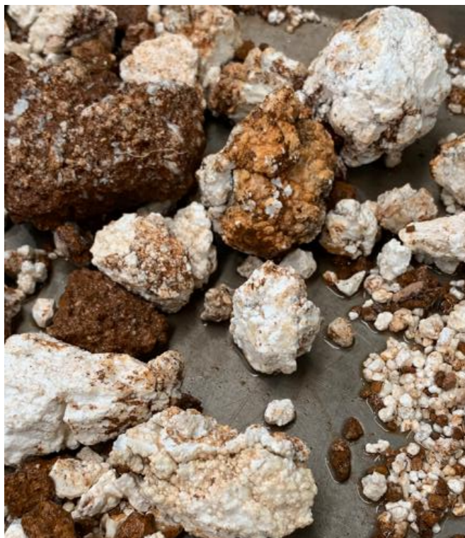
Figure 11. Coarse surface material containing calcite, magnesite and gibbsite.
