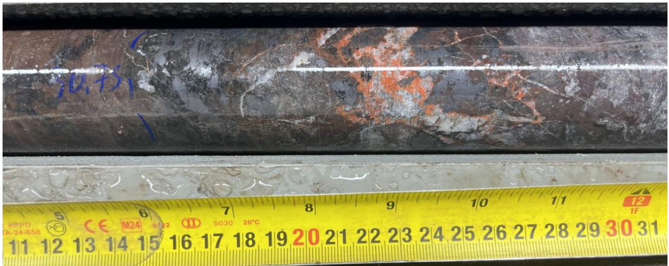
Figure 01- Photograph of coarse-grained chalcocite mineralisation within a basaltic peperite crosscut by quartz-calcite veining. DAN26052 30.75-30.90m.
