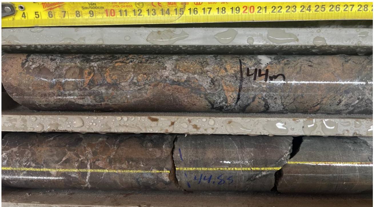
Figure 02 - Photograph of chalcocite cement within a breccia intersected in DAN26052 between 43.80 and 44.85m downhole. Chalcocite is observed forming around the edges of clasts within the breccia.
