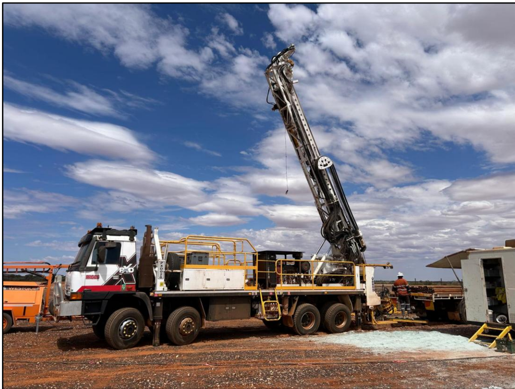
Figure 1 Diamond Drilling at Beatty Park Sth.
