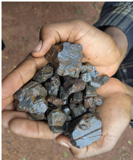
Figure 2: Rutile nuggets returned analysis at 98.4% TiO 2 .
