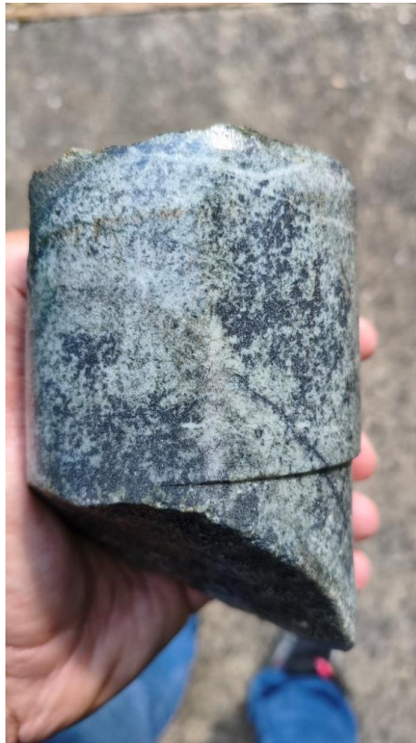
RAV26011 core: pervasive silicification with bismuthinite-pyrite in the 1 m @ 37.8 g/t Au interval.
