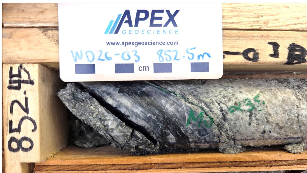
Figure 11: Very strong visual molybdenite (blueish-grey)-quartz-pyrite veining in NQ drill core from approximately 852.45m downhole in drill hole WD26-03. Laboratory assays for this interval are pending.
